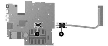
3. Reverse this procedure to replace the heat sink. Replace the thermal material that ships with the replacement heat sink.
